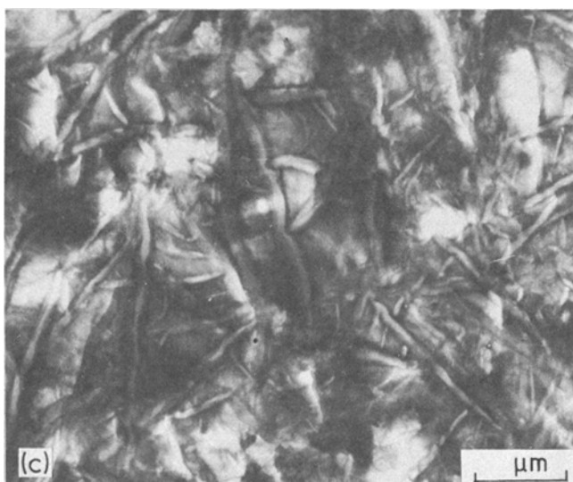
Figure 9 Detail in stained Hifax samples: (a) lamellae which commenced to crystallize as thick lamellae of the hexagonal structure and continued to grow as thin orthorhombic laminae, (b) thin lamellae with tapered growth edges which crystallized directly into the orthorhombic phase and (c) lamellar impingements in a chain-extended sample.
